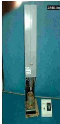
The Civilab EZIPAC soil compactor is designed to produce compaction samples without sacrificing the accuracy of hand compaction. The EZIPAC will perform standard and modified tests in either one litre, two litre or 2.4 litre compaction moulds conforming to AS1289.CBR Samples can also be compacted.
